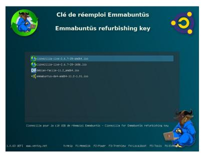
In the above window, you can run the refurbishing script with either 64-bit or 32-bit Clonezilla, and you will get one of the windows below to run the cloning script :
