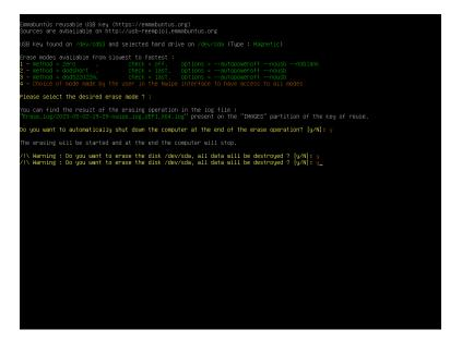
After validation of the choice, the Nwipe utility is launched and keeps the user informed with the progress of the erasing operations :
