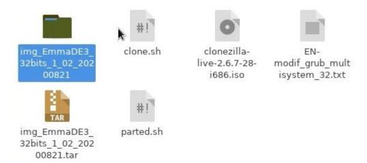
In order to copy files and folder, you need the admin rights, because the second partition is of type ext4 and is mounted by default in write mode only. So, to make it simple, you launch Thunar in "root" mode and you copy-paste the relevant objects.
