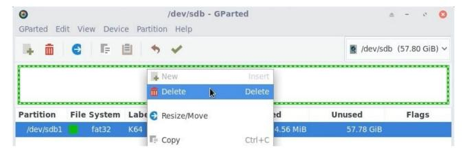
Create a vFat partition of 4,500 MB to host Multisystem (it is possible to define a partition of a smaller size, see the tips at the end of this documents):
