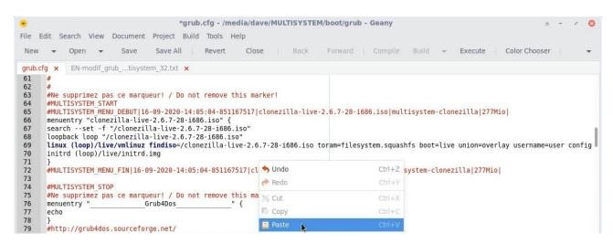
Here after the resulting grub.cfg file, with its new entry:
